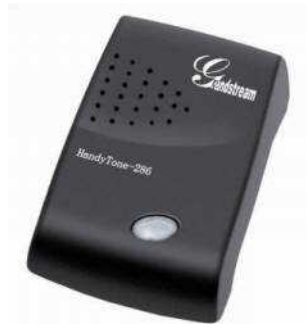
Figure 3 - An ATA adapter
